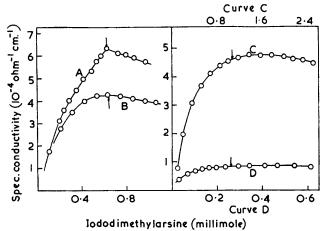
conductimetric plot in the vicinity of the end-point. Evidence for the formation of the chloride, which could not be isolated in a pure state, was obtained only from a conductimetric titration. Similarly, unstable salts were formed from triethylphosphine and iododiphenyl-antimony and -bismuth, but in neither instance could a pure product be isolated.
